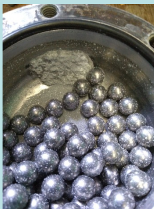
Fig. 1. Photo of lump formed by Al powder PA-4 and Ga-In-Sn eutectic in mill.
